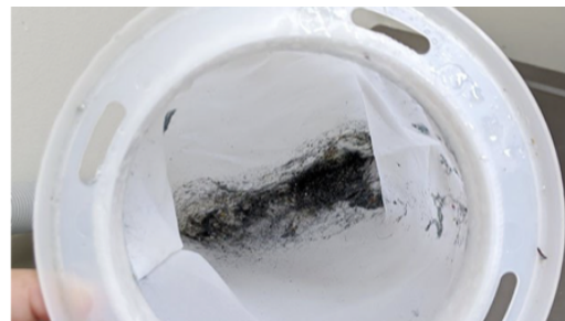
Microfibers shed from washing machines captured in a 100 \mu m filter
